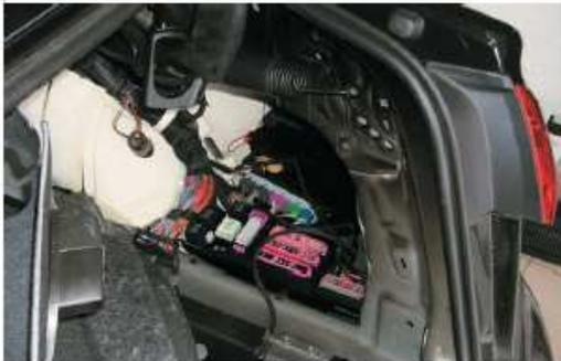
Remove the two lashingeyes in the right floor plate. Pull out the stainless steel faceplate of the back door lock. Remove the fender side-covering. The Wabco-Ecu in a black box with 5 plugs. The plugs with 15 and 9 pins, delivered with the lowering, are adapted here. The brown plug with 16 pins is adapted to the park-assistent ECU, 2 brown plugs and one black, located just above the suspension ECU.
